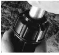
**6. Fully Installed**The fitting is fully installed when the nut butts against the flange of the body.
