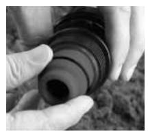
**2. Position the Connection Kit**Take the appropriate connection kit and place it in the body of the fitting with the tapered end pointing outwards.
